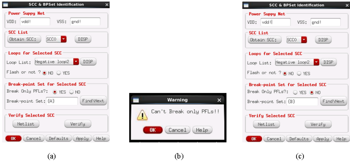
Figure 6.8: Select Break Points: (a)Only Break PFLs; (b)The Warning for “Can’t Break Only PFLs”; (c)Break Both PFL and NFL
