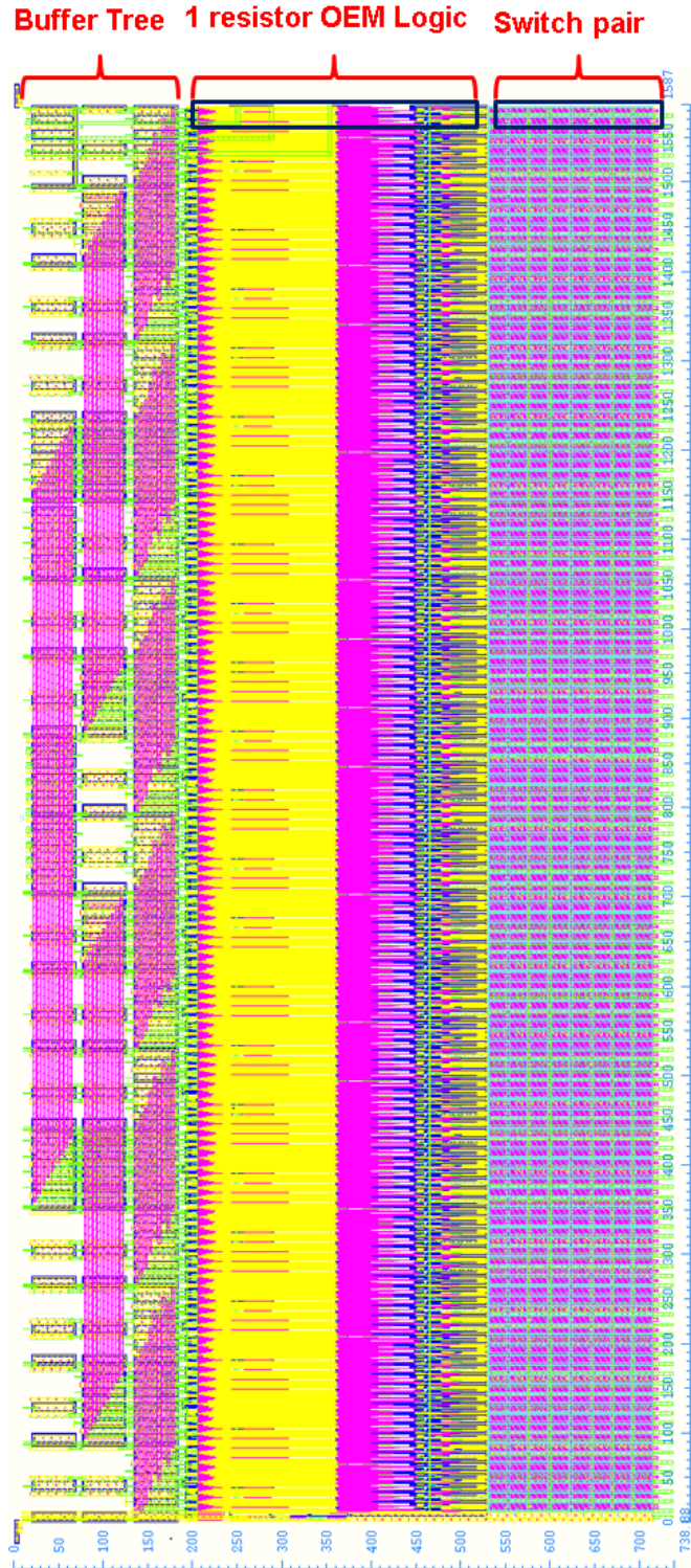
Figure 3.9: Layout of MSB Buffer Tree, Digital Circuits and Switches
